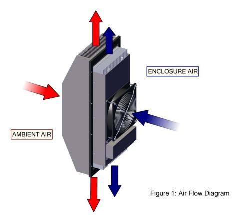
NOTE: Condensate may be formed on the internal heat sink inside of the enclosure when operating in the cooling mode. Mounting location should take into consideration dripping condensate or condensate being entrained with the air circulated inside the enclosure that would possibly damage equipment.
