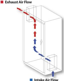
The Ice Qube Washdown Filter Fans are designed to eliminate the threat of water damage to enclosed electronics, even in work areas that require direct hose wash down. A powerful blower draws 155 / 310 or 250 / 500 CFM filtered ambient air into the enclosure to cool the enclosed electronics.
